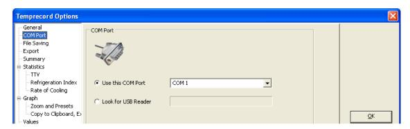
**10.** Place a Temprecord data logger into the Reader then press '**Space Bar**'. This should access the data logger and display Summary screen with Serial Number and type of data logger at the top.
